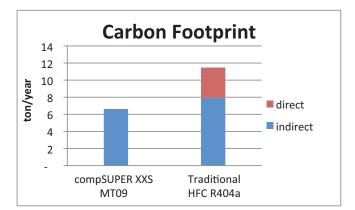
The calculation is based on Pack Calculation II ver. 3.05 with a Danfoss MTZ50-4 piston compressor, using HFC refrigerant against the XXS MT09 unit with a dimensioning ambient temperature of 30°C and an evaporator capacity of 9 kW at -8°C.
