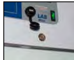
Door lock with keys as standard, USB port optional
