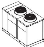
Multicompressor pack systems with built-in condenser
