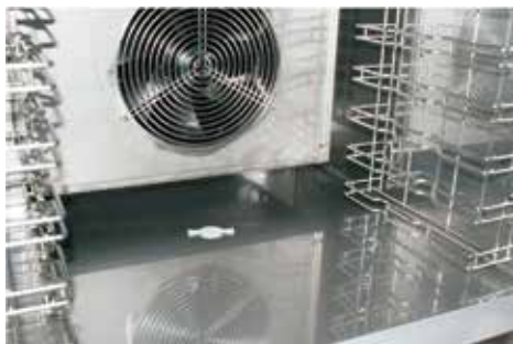
Washing water drain with cap
